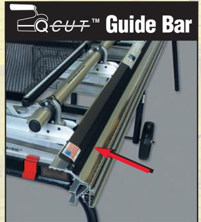
Works with Q-Cutter and Q-Cutter Stop. Lines up pencil marks to cutter wheels.
