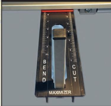
Adjustable measuring device designed for repeat cuts and bends. Simply set distances. No pencil needed. Automatically stack all cut pieces on maximizers. Coil cannot drop to the ground. Sold in sets of 4.
